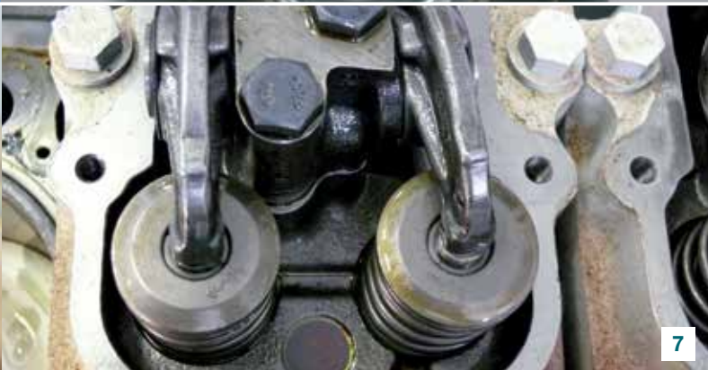
1. MAN E 2842 LE 302 V12 Piston with ring grooves; 2. GE Jenbacher J 412 V16 Bearing shells; 3. MWM TCG 2016 V12 Piston with ring grooves; 4. MWM TCG 2016 V12 Valve train; 5. GE Jenbacher J 312-1 V16 Piston with ring grooves; 6. GE Jenbacher J 312 V12 Sparking plugs; 7. MTU Onsite Energy AB 3066 L4 V6 Valve train; 8. MTU Onsite Energy AB 3066 L4 V6 Inlet and exhaust valve.
