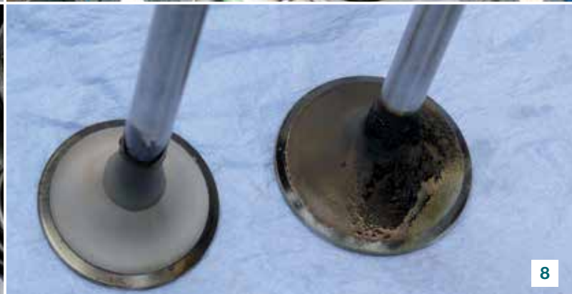
1. MAN E 2842 LE 302 V12 Piston with ring grooves; 2. GE Jenbacher J 412 V16 Bearing shells; 3. MWM TCG 2016 V12 Piston with ring grooves; 4. MWM TCG 2016 V12 Valve train; 5. GE Jenbacher J 312-1 V16 Piston with ring grooves; 6. GE Jenbacher J 312 V12 Sparking plugs; 7. MTU Onsite Energy AB 3066 L4 V6 Valve train; 8. MTU Onsite Energy AB 3066 L4 V6 Inlet and exhaust valve.
